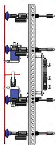
Pneumatic brake suspensions can absorb an ejection stroke and then be locked in place for degating as shown in the above application.
