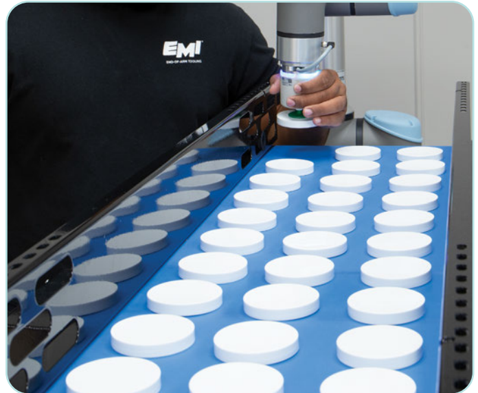
Ideal for automated handling of small parts, such as pick-and-place applications with a single suction cup, as shown above.
