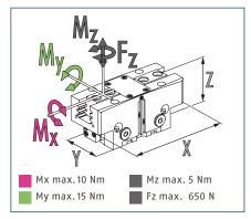
The indicated moments and forces are statical values, apply for each base jaw and may appear simultaneously. Loads may additionally occur to the moment produced by the gripping force itself.
