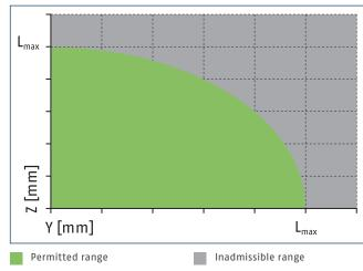
$L^{\text{max}}$  is equivalent to the maximum permitted finger length, see the technical data table.
