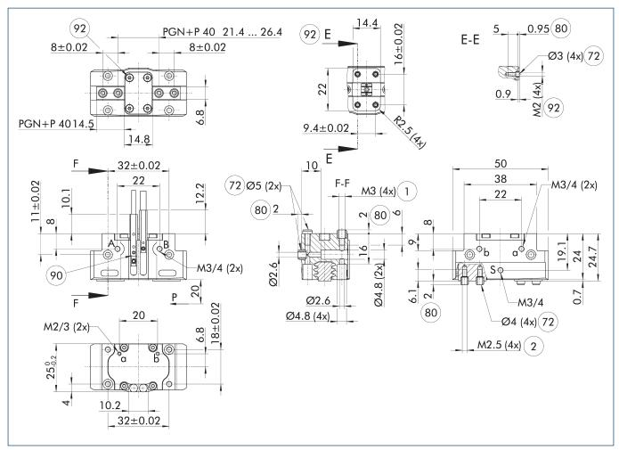
The drawing shows the gripper in the basic version with closed jaws, without dimensional consideration of the options described below.
